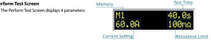
Follow the setup procedures to set the desired parameters. The display will show the Ground Bond test settings depending:
